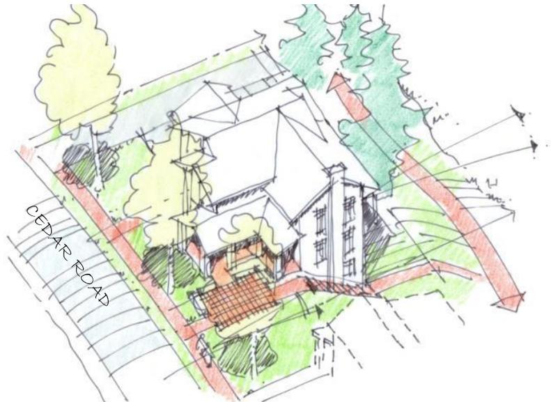
Example of how topography could be used to support of third storey within the roof on the downslope side of a parcel.
