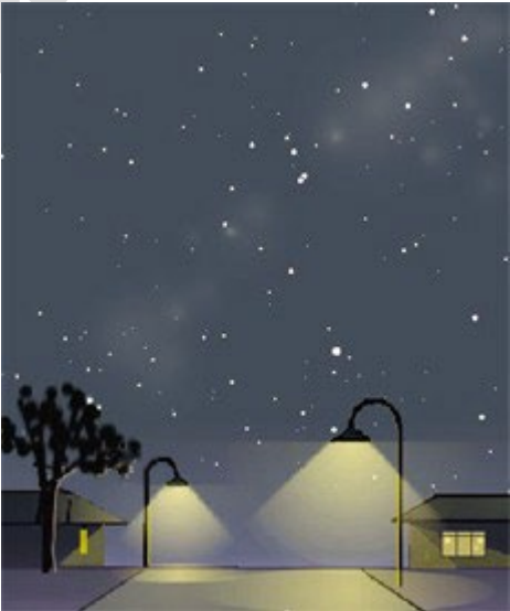
Example of full cut-off light fixtures with direct light below the horizontal plane reducing light pollution and protecting the night sky
