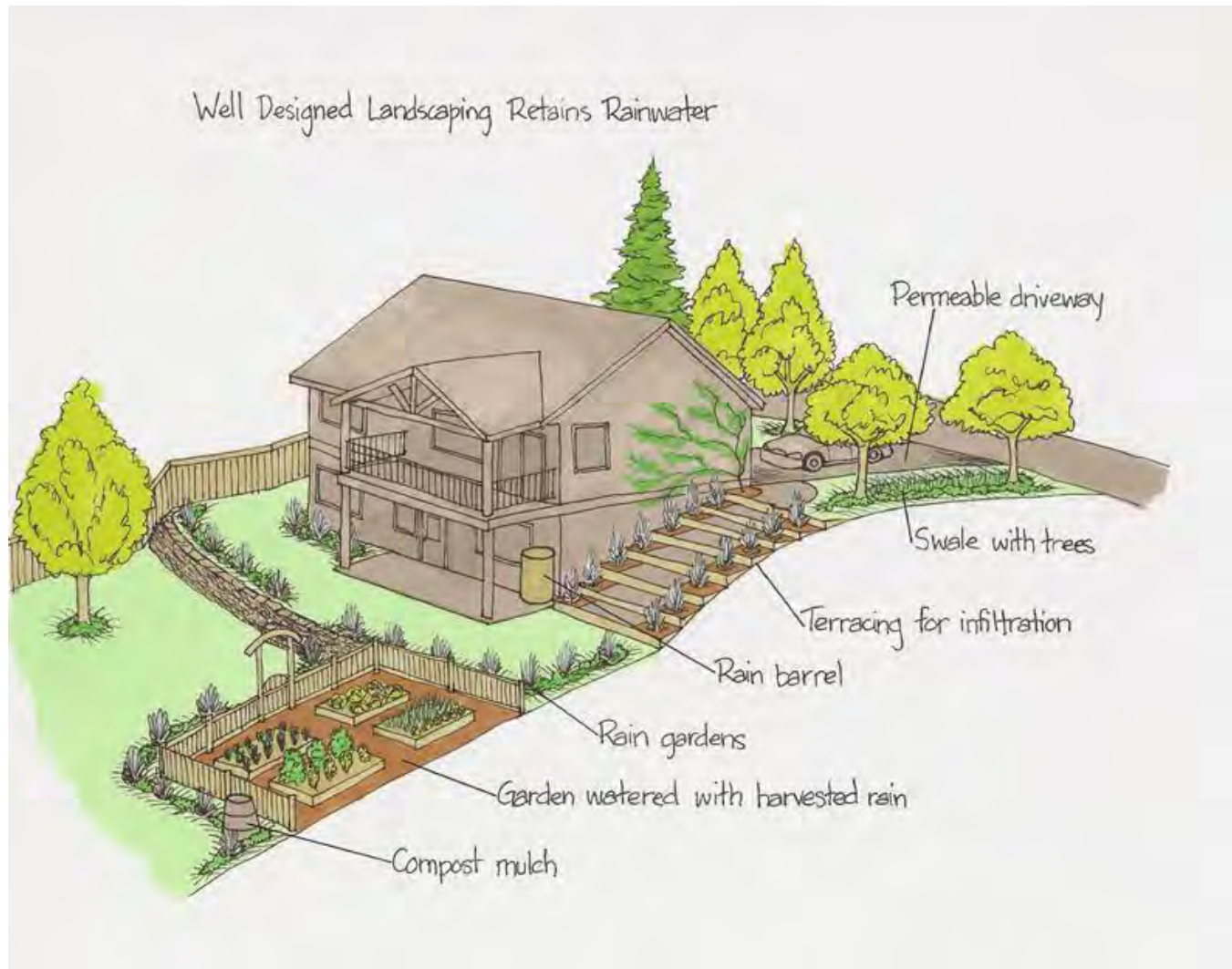
Figure A157. A well designed residential property with rain gardens and swale. Drawing provided by Larratt Aquatic Consulting and illustrated by Rebekah Massey.
