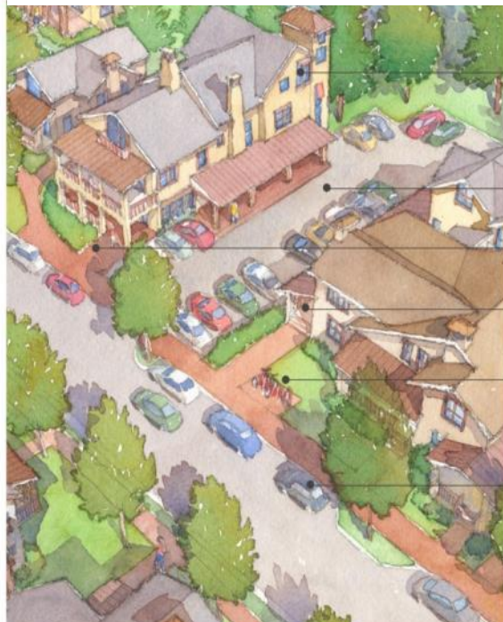
Illustration of desirable design elements such as mixed on and off street parking and shared travel ways between developments.
