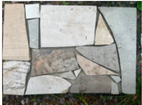
Garden paving slabs from broken tile
