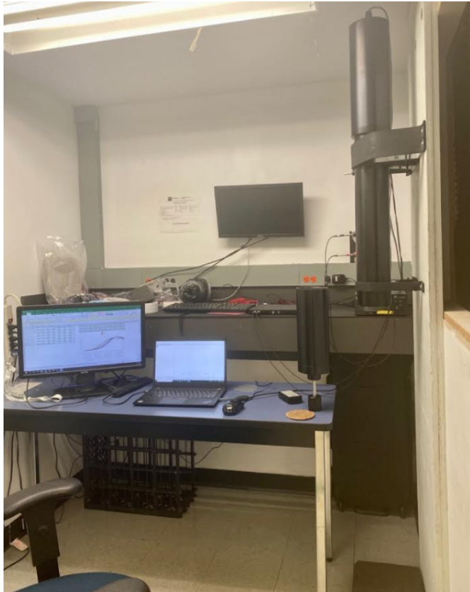
Figure 1 Impedance Set-up to determine absorption of shreds
