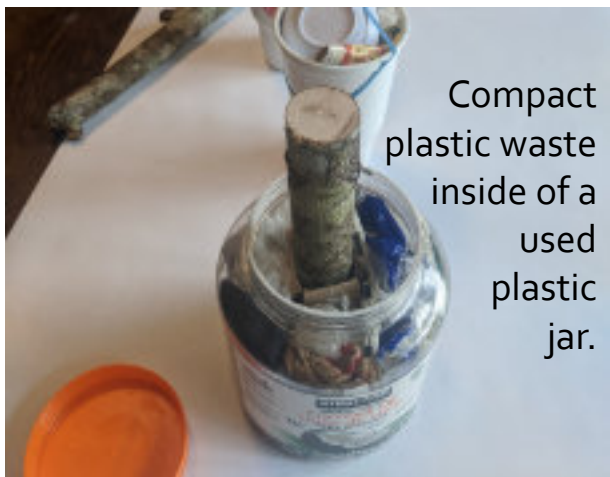
Wooden stakes create a rebar space
